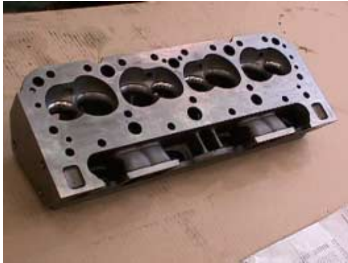
Fig. 1: A machined V8 "Iron Lightning" cylinder head cast and machined at TF.
